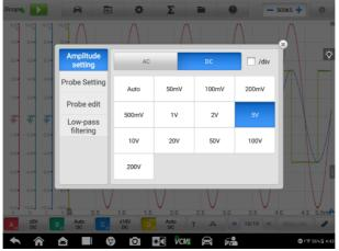
Figure 8-41 Amplitude Setting Screen (DC 5 V)
