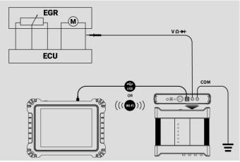
Figure 8-93 Actuator Drive Connection Diagram
