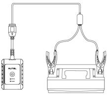
Figure 10-4 Battery Tester Connection Example 2
