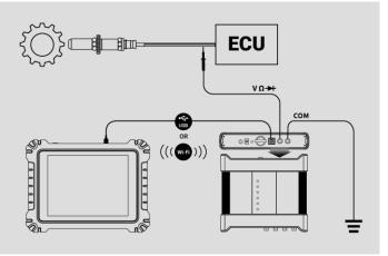
Figure 8-94 Square Wave Connection Diagram
