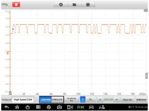
Figure 8-122 Communication Line Button Screen
