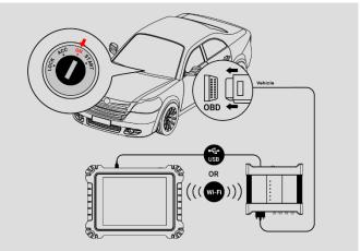
Figure 8-107 Connection Diagram
