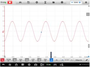
Figure 8-50 Trigger Point Screen
