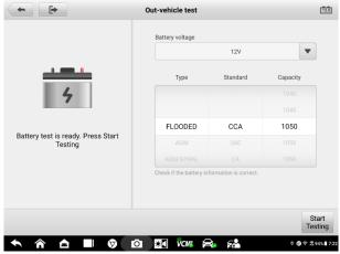
Figure 10-10 Out-vehicle Test Screen
