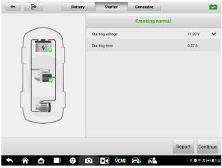
Figure 10-8 Starter Test Result Screen
