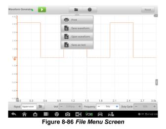
♦ Print — tap to create and print a temporary PNG picture of the current waveforms.
