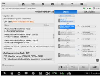
Figure 5-21 Repair Assist Screen 4
