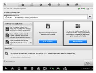
Figure 5-17 Repair Assist Section
