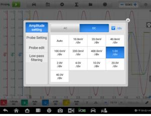
Figure 8-42 Amplitude Setting Screen (DC 1.0 V/div)
