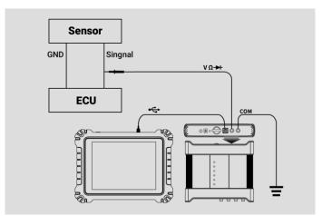
Figure 8-96 Triangle Waveform Connection Diagram
