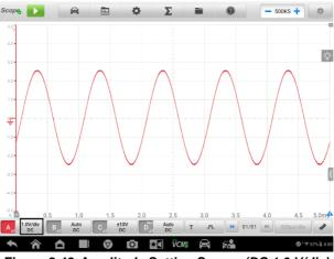
Figure 8-43 Amplitude Setting Screen (DC 1.0 V/div)
