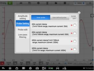
Figure 8-44 Inner Probe Setting Screen
