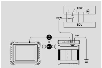
Figure 8-92 DC Voltage Connection Diagram
