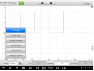
Figure 8-91 Signal Mode Setting Screen
