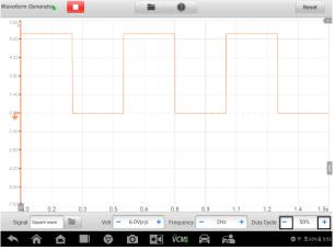
Figure 8-104 Duty Cycle Setting Screen 1
