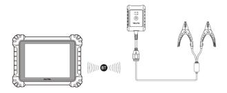
Figure 10-3 Battery Tester Connection Example 1
