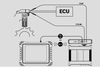
Figure 8-95 Square Wave (X+Y) Connection Diagram
