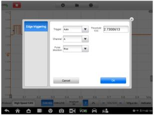
Figure 8-127 Trigger Mode Screen
