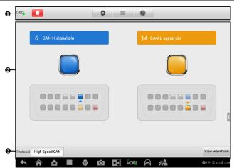
Figure 8-110 Bus Inspection Screen
