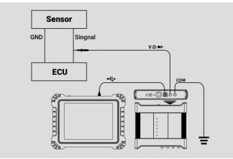
Figure 8-97 Arbitrary Waveform Connection Diagram
