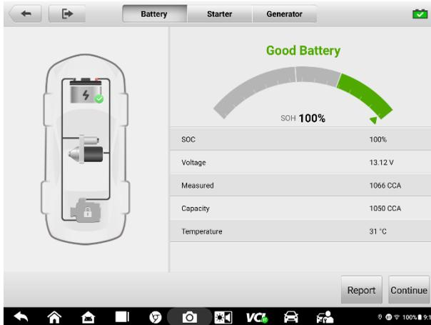
Figure 9-6 Battery Test Results Screen
